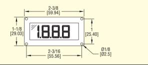
**The Model DPMF Flush Mount LCD Digital Panel Meter** offers high performance and low cost in a compact package. This meter is designed with a 3-1/2 digit, high contrast LCD display. The unit is powered by a 4 to 20 mA DC control loop input. Standard features include adjustable span and zero, and field-selectable decimal point position. The flat pack of the panel meter allows for the instrument to be mounted to any flat surface.
