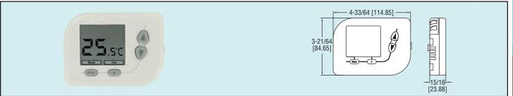
The Model PLVT1 Compact Digital Thermostat with Heat Pump directly controls the furnace, small boiler, air conditioner, circulator fan, and heat pump in commercial or residential buildings. A large easy to read LCD display shows the current temperature and the operating mode. In case of a power outage, the thermostat can be operated off batteries. In order to reduce the need to switch modes for different seasons, the thermostat can be set to automatically switch between heating and cooling.
