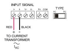
Measuring Current with PDA6405-100 Current Transformer and PD6400 digital panel meter.
