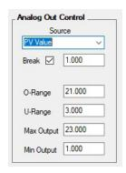
**Source:** Source for generating the 4-20 mA output (e.g. PV)
