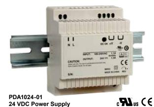
Input Voltage 85 ~ 264VAC 120 ~ 370VDC **Output Voltage** 24 VDC; ±10% 1.5A rated current
