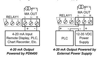
The internal 24 VDC power supply powering the analog output may be used to power other devices, if the analog output is not used. The I+ terminal is the +24 V and the R terminal is the return.
