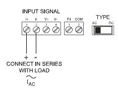
**Current Input Wiring Example with AC Switch Selected**
