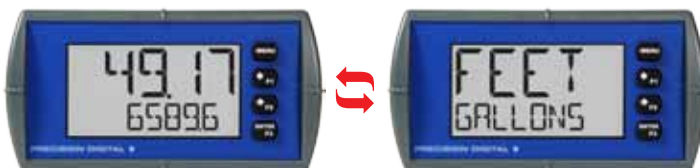
Feet Value on Top Gallons Value on Bottom
