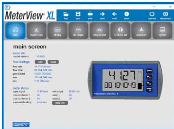
▲ The main screen displays an image of the connected meter and includes various information about this meter, such as model number, readings, and status.
