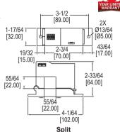
The Series CCT40/50 Current Transformers are a low cost alternative for measuring power and monitoring the operation of fans, pumps, or other equipment. For use on existing installations, split core models can be installed without disconnecting cables. Each model offers three jumper selectable ranges and a choice of three different outputs.
