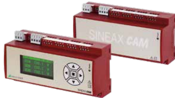
Fig. 1. SINEAX CAM in top-hat rail housing.
