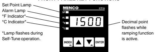
The 1500 Series controls have one display. The display must occasionally switch to show a complete message or menu item and its value. The normal display shows just the temperature and does not switch. While showing a menu item, the display will alternate between the menu item and the item value. If the UP arrow, DOWN arrow, or ENTER keys are pressed, the display immediately switches to display the item value.
