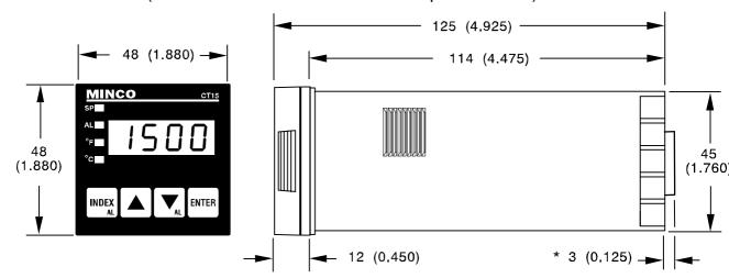
Panel cutout for all models 45 mm X 45 mm (1.775" X 1.775"). Allow for 13 mm (0.5") clearance at the rear of instrument.
