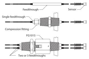
Disadvantages: Location on leads must be predetermined. Cannot be repaired.
