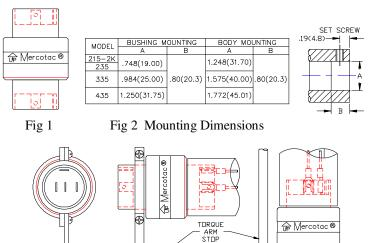
Fig 3 Floating Torque Arm Examples
