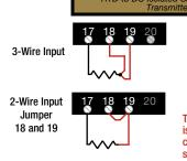
Cu 60/75°C conductors 14 AWG max.
