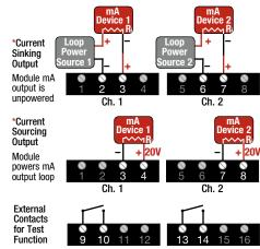
To avoid damage to the module, do not make any connections to unused terminals
