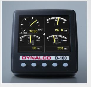
D-100 CANbus monitor offers J1939 compatibility for displaying engine performance parameters as well as providing over/under speed threshold protection. The D-100 can also monitor and display various types of inputs to help measure parameters such as temperature, pressure, and RPM. Plus it can send output signals to trigger controls via 4 independent relays.
