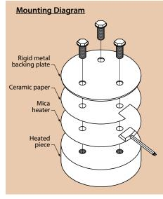
mm) thick stainless steel with pre-drilled holes matching the bolt pattern of the specified model. These backing plates do not have cut out areas for the lead bulge and may require modification.
