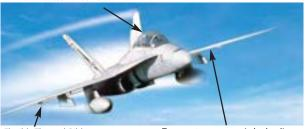
Flexible Thermal-Ribbons sense wing surface temperatures for wing surface de-icing.
