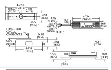
The Model UFM Compact Ultrasonic Flowmeters are economical, clamp-on, ultrasonic flowmeter. The Model UFM implements the transit-time difference to measure flow rates in pipes and can measure velocity and flow in pipes with outside diameters ranging from 0.98 to 4.62" (24.89 to 117.35 mm). This model comes with a volume pulse and 4 to 20 mA flow rate output.
