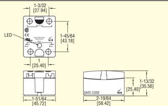
Series 62 Hockey Puck Style Solid State Relay features a terminal cover and LED status indicator. The optically coupled circuitry isolates the input terminals from the output terminals to give the relay 100% pure solid state performance.
