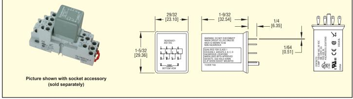
**The Series 782H Hermetically Sealed Ice Cube Relay** is suitable for switching up to four circuits in a hazardous environment. It features a hermetically sealed housing and a safety seal to withstand a wash-down. The plug-in socket is easy to mount and remove from crowded DIN rails.
