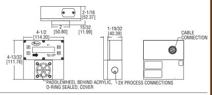
The **SERIES DPW** Digital Paddlewheel is an economical choice for applications where remote or local liquid flow measurement is desired. This Series offers two programmable totalizers via the optional LCD and RS-232/RS-485 interface, two optically isolated flow pulse outputs, and selectable 0 to 5 VDC or 4 to 20 mA flow outputs (optional temperature).
