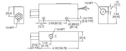
The Series P1 Brass Flow Switch utilizes a piston-type design for accurate detection of excessive or insufficient liquid flow rates. The switches have preset actuation points from 0.10 to 1.5 GPM for liquid flow.
