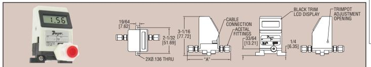
Series TFP-LI Liquid Turbine Flow Meters are suitable for a wide variety of industrial. commercial, and laboratory flow applications. These meters utilize a turbine wheel and electro-optical detection to convert flow rates into a linear 0 to 5 VDC output signal for recording and data logging. A 3-1/2 digit LCD informs the user of the actual flow rate. A power adapter or mating cable assembly is required for operation.
