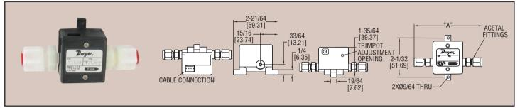
Series TFP-LP Liquid Turbine Flow Meters are suitable for a wide variety of industrial, commercial, and laboratory flow applications. These meters utilize a turbine wheel and electro-optical detection to convert flow rates into a linear 0 to 5 VDC output signal for recording and data logging. Couple this unit with a Series TM2 Flow Totalizer for a remote flow monitoring display. A power adapter or mating cable assembly is required for operation.
