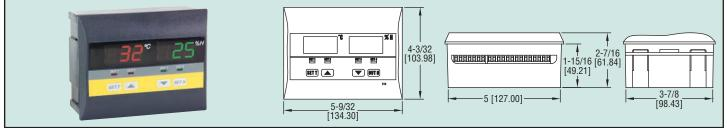
**Simultaneously measure and control** temperature and humidity with the Series THC Temperature/Humidity Switch. The unit offers a 3-digit red display for temperature indication and a 3-digit green display indicating humidity. The Series THC is equipped with four independent relays, two for temperature control and two relays for humidity control.
