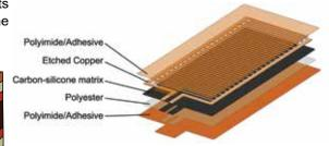
SmartHeat incorporates the functions of sensor, controller, and heater into a compact, thin-film form factor.
