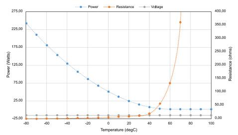
Polymer resistance increases to reduce power draw as target temperature is reached.
