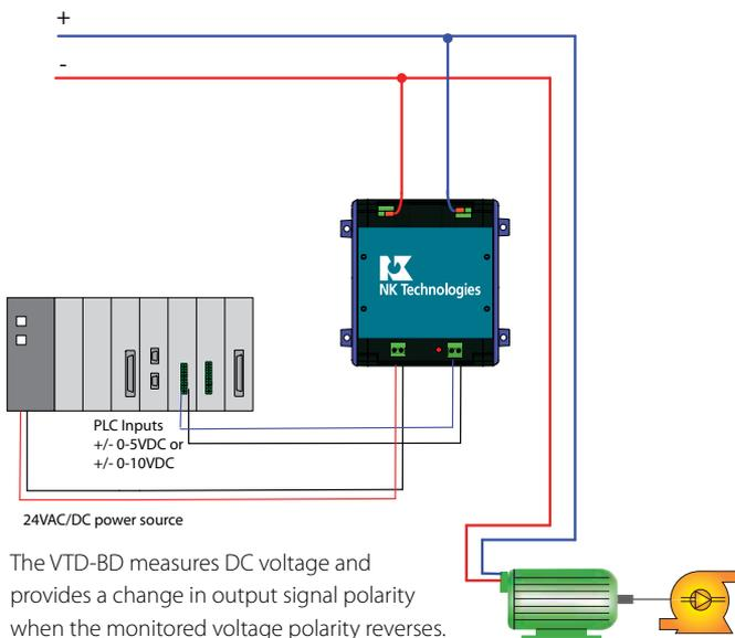
The VTD-BD measures DC voltage and provides a change in output signal polarity when the monitored voltage polarity reverses. Positive on upper right terminal creates a positive output signal; positive on upper left terminal creates a negative output signal.
